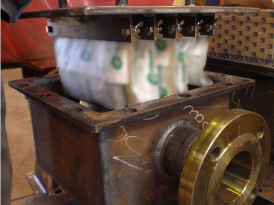
Figure 7: An example of a plenum that could be installed to introduce VpCI A to a sprinkler system.
